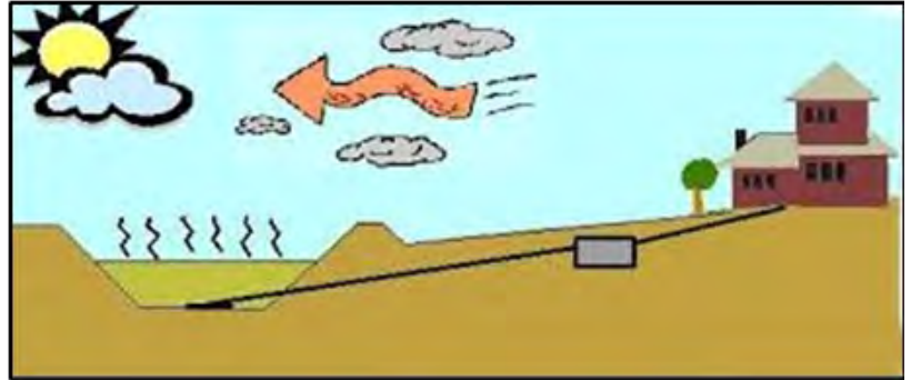
A diagram of how an on-site septic system works when incorporating a lagoon in place of a leach field
