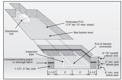
Figure 5. View of a typical absorption bed.
