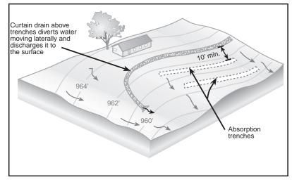
Figure 11a. View of curtain drain location.
