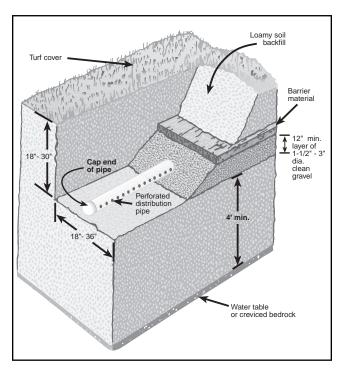
Figure 6. View of typical trench construction dimensions.
