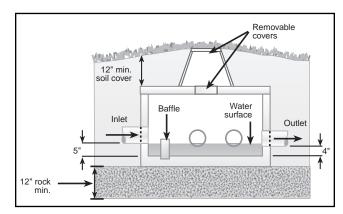
Figure 7. Section view of a distribution box, or D-box.
