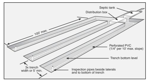
width apart, or a minimum of 5 feet on center, whichever is greater. Make the trench bottoms level, and fill the trenches at least 12 inches deep with  $1\frac{1}{2}$ - to 3-inch diameter clean, washed gravel or crushed stone. If limestone is used, all fine materials should first be screened out to prevent clogging the system. Place at least 6 inches of the gravel below the perforated pipe and 2 inches over the pipe.
