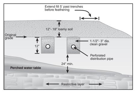
Figure 12a. Shallow placement of absorption trenches.
