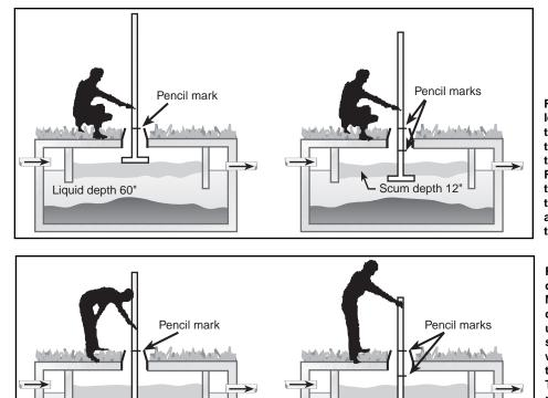
Figure 14a. Measuring the scum level in the septic tank. Left: Lower the bottom of the board to the top of the mat of scum. Mark the stick at the top of the tank opening. Right: Force the board all the way through the mat. Bring it back until you feel the bottom of the mat. Mark the stick again. The distance between these two marks is the scum depth.
