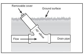
Figure 3b. PVC pipe cleanout for drain pipe.
