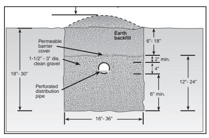
Figure 10. Section view of an absorption trench.
