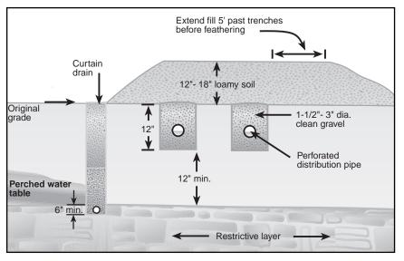
Figure 12b. Modified shallow placement of absorption trenches.
