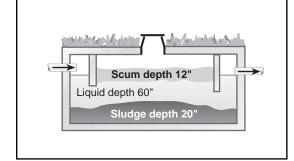
Figure 14c. Determine if the tank should be cleaned. Add the scum and sludge depths. If this figure is more than half the liquid depth, clean the tank. The maximum available liquid depth in this example is 60 inches. The scum depth is 12 inches and the sludge depth is 20 inches — a total of 32 inches. Since this is more than half of the maximum liquid depth, this tank should be cleaned.
