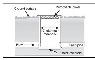
Figure 3a. Manhole cleanout for drain pipe.
