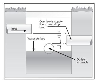
Figure 9. Section view of a stepdown or drop box.
