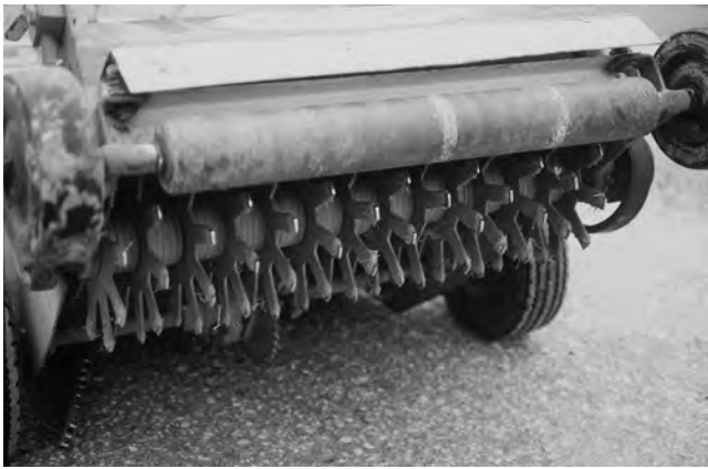
Figure 4. Verti-cutters and de-thatchers, with multiple blades set low enough to touch the soil surface, prepare an excellent seedbed and create good seed/soil contact for turfgrasses.
