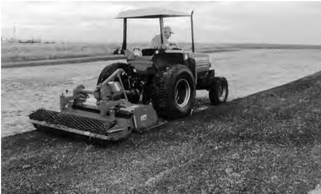
Figure 1. This roto-dairon prepares the seedbed for turfgrass establishment and also maintains the grade in a firm bed.
