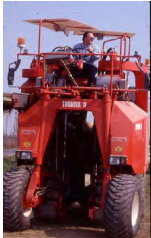
Figure 6. The overhead TRINOVA vertical head unit, specifically designed for the MFC.
