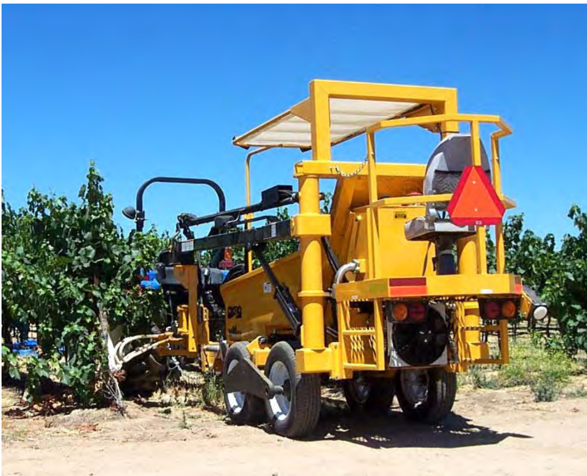
Figure 6. Korvan™ Vineyard System chassis equipped with grape thinning attachments for bottom thumper fruit thinning on 2-ft lyre and quadrilateral-trained vines. Shown working in Vitis vinifera at French Camp Vineyards, Santa Margarita, Calif. (Photo courtesy of OXBO International Corp., Clear Lake, Wis.)
