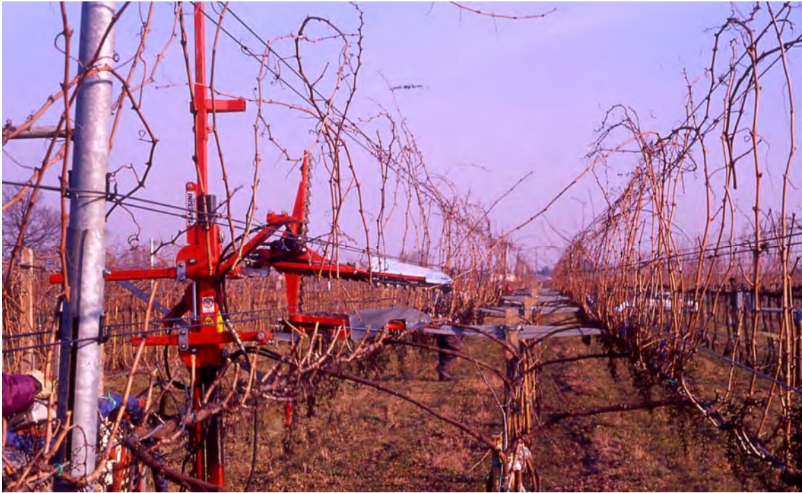
Figure 10. The COMBI can be pruned with the same multiple-blade TRIMMER unit used for DC.
