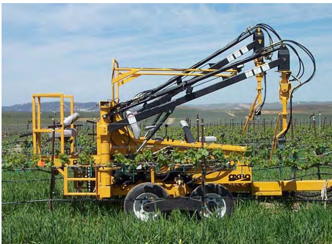
Figure 5. Korvan™ Vineyard System chassis equipped for shoot thinning. The speed of the tractor pulling the chassis and the speed of the thinner paddles can be adjusted so that the thinner leaves the desired number of shoots per meter of cordon, depending on cultivar and vigor. (Photo courtesy of OXBO International Corp., Clear Lake, Wis.)
