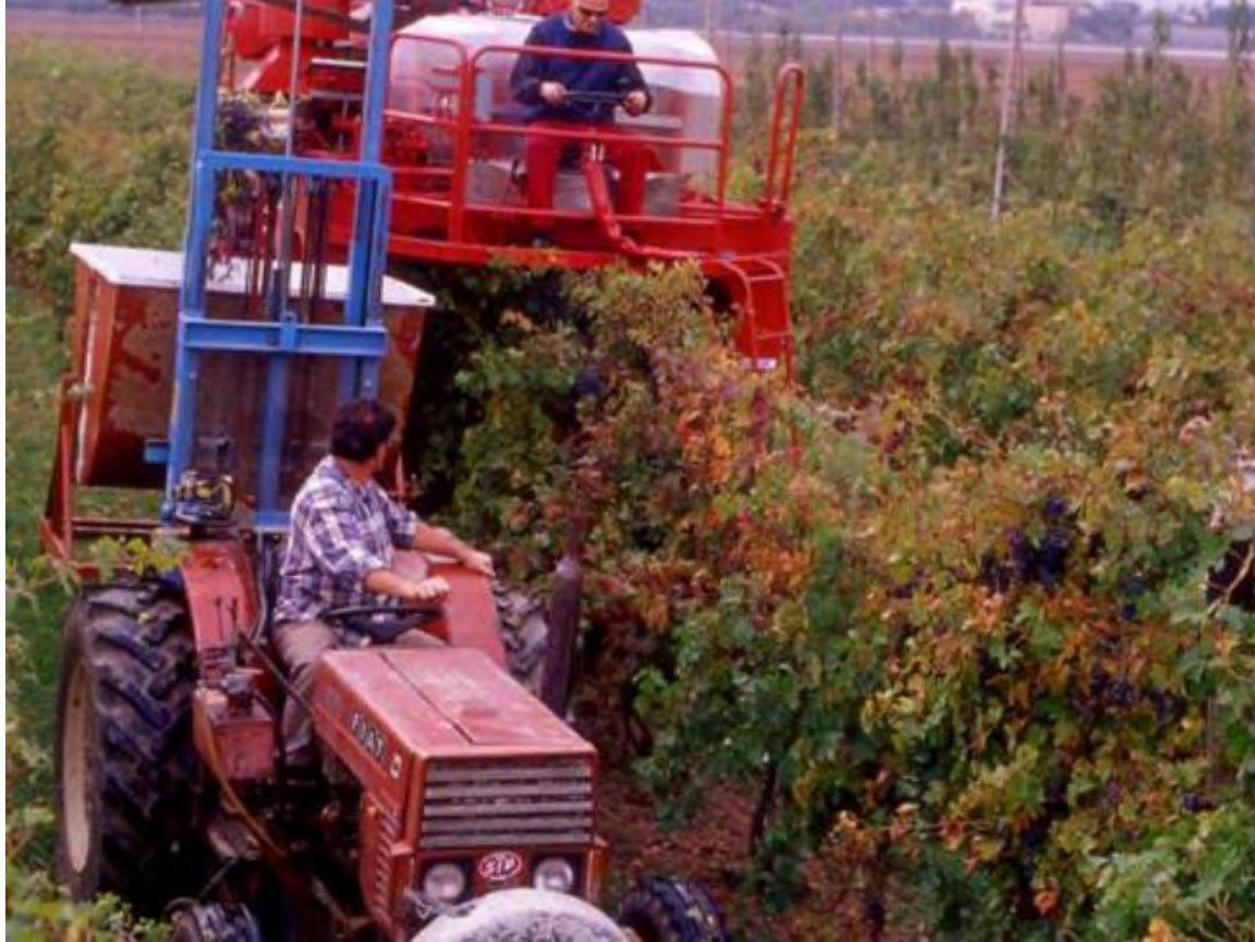
Figure 13. The SMPH can readily be harvested by conventional horizontal slapper-head units.
